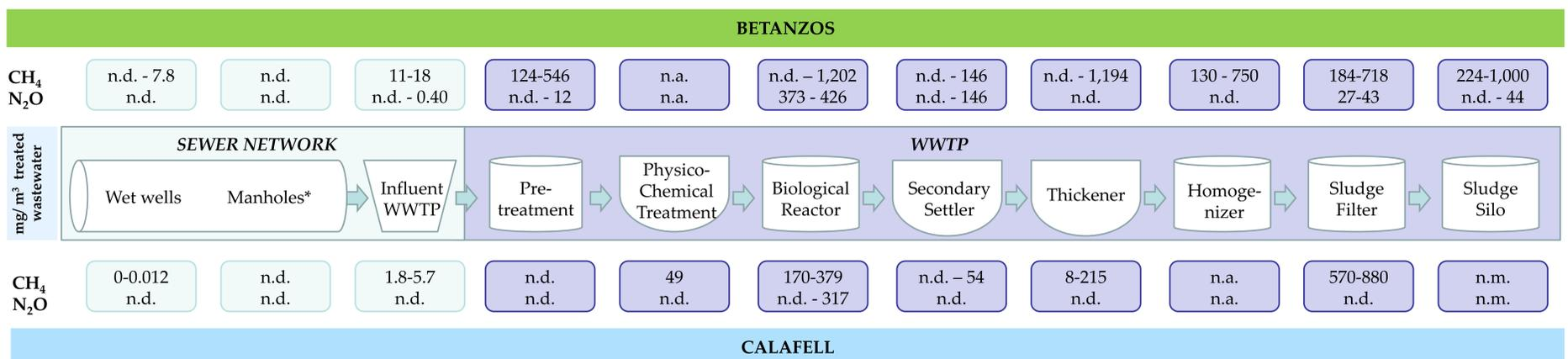
Figure 2. Range of direct GHG emissions measured in different sites. The results are an average of the summer and winter sampling campaigns. n.d.: not detected Detection limit (ppm<sub>v</sub>)= 2; n.a.: not available, treatment step not present in the WWTP; n.m.: not measured
